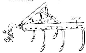
When assembling for in-between row cultivation, the extra shank must be mounted to the center of the cultivator, using the same hole and bolt used to fasten tie bars to pull bar, as shown. Set all shanks to run straight in the direction of travel.
