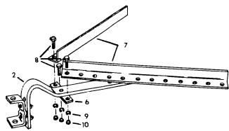
FIG. 3. Assemble tie straps (11) to pull bar with a ½" x 2" hex bolt (12), lock washer (13), and hex nut (14). Align the tie bars with appropriate holes on each of the frame angles. Note: The holes used should be selected to create the desired width of cultivation. The forwardmost holes provide the widest path of cultivation, and the rearmost holes the narrowest. Secure the tie bars to the frame angles with ½" x 1½" hex bolts (15), lock washers (16), and
